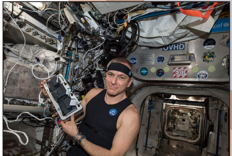
CSA astronaut David Saint-Jacques tries the Bio-Monitor - an innovative smart-shirt system designed to measure and record vital signs [Courtesy: CSA/NASA, 2019]
