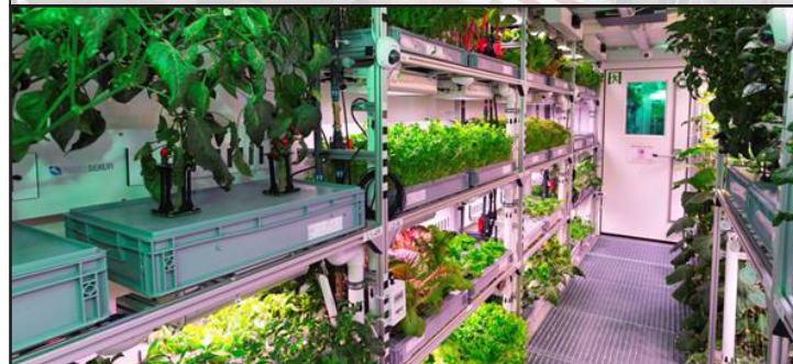
The Future Exploration Greenhouse is located at an Antarctic research base. The University of Guelph and other international partners are using this test facility to develop plant cultivation technologies for space [Courtesy: DLR, 2017]
